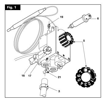
Remove lock screw (pos. 19 fig. 1) from the pressure intake tube and connect the gauge hose: once measurement is complete, replace the screw and do a seal check using a leak detector spray.
