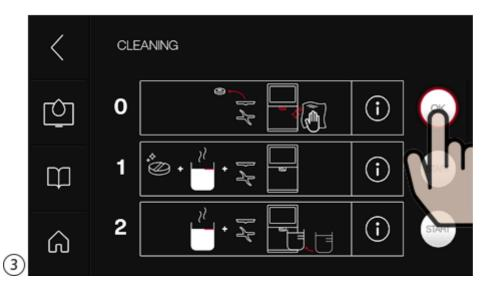
Clean the tool coupler with a soft, non-abrasive brush and cloth. Select "OK" to check off the first cleaning cycle as complete.
