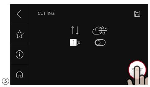
Press "Start" to start the cutting process.
