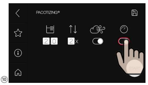
Press the Jet® Mode button if you would like to use a faster processing time (processing time 90 seconds). This automatically changes the number of repeats to 2, which can be changed later.
