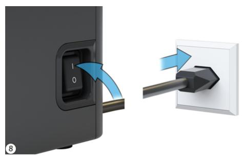
Carefully set the device upright. Plug the device in and turn it on.
