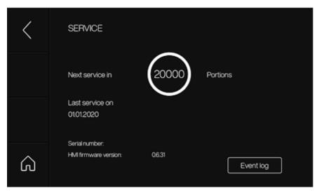
Service: Displays the time to next service, date of the last service, and log data. Firmware version is displayed.
