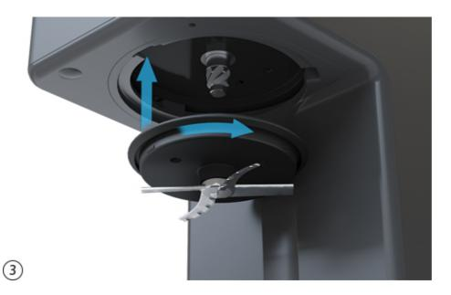
Attach the combination of the spray guard, preliminary scraper, and pacotizing® blade to the tool coupler on the pacotizing® shaft. The pacotizing® blade is properly attached when it holds tightly to the tool coupler.
