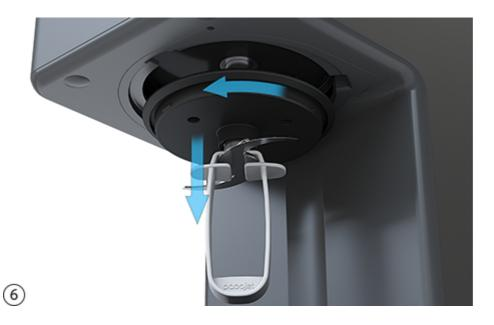
Remove the coupe set knife with the help of the cutter tongs.
