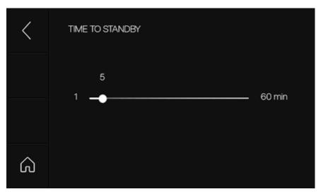
Standby: The device switches to standby mode after I to 60 minutes.
