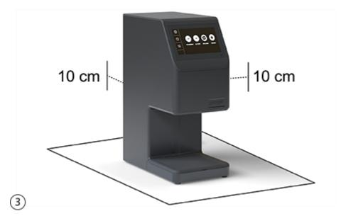
Place the device on a firm, flat surface at a distance of at least 10 cm to any other object.
