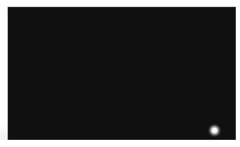
• Note: If the device is not used for several minutes, it switches over to standby mode. The display will turn off. A white LED will light up on the right side under the touchscreen. The device switches back to operating mode when the touchscreen is touched. The standby time can be changed in "SETTINGS."
