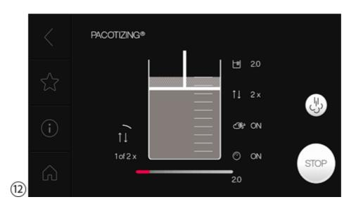
During the pacotizing® process, the selected parameters as well as the processing progress are displayed.
